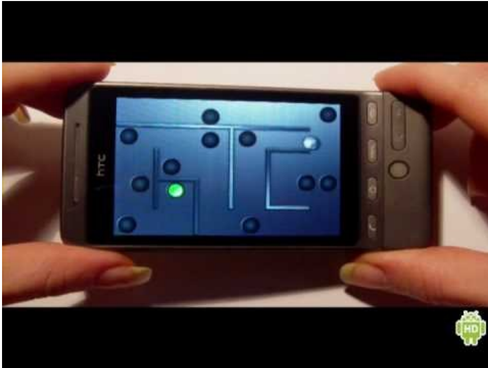
Figure 1. A picture of the Android mobile HTC Hero with the game Teeter. The mobile is being tilted and the teeter ball is controlled by the tilt. 4
