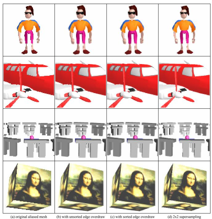
Figure 6: Edge overdraw results. Images (a-c) are rendered at 100x100 resolution, while (d) is rendered at 200x200 and averaged down.
