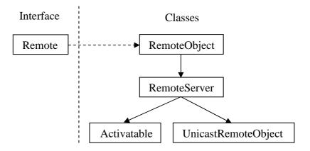
Figure A-2. Interfaces and Classes in the *java.rmi* package.
